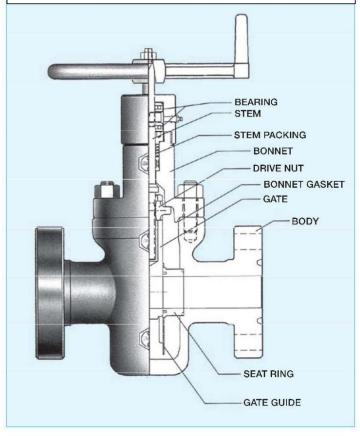
Sizes: 2 1/16" to 4 1/16" Pressure Rating (Psi): 10000, 15000 Design: API 6A. Ends: RTJ, THRD. Style: Slab. Materials: AA, BB,CC,DD,EE,FF TEMP (°C):-46~343. PSL-3. PR-2
